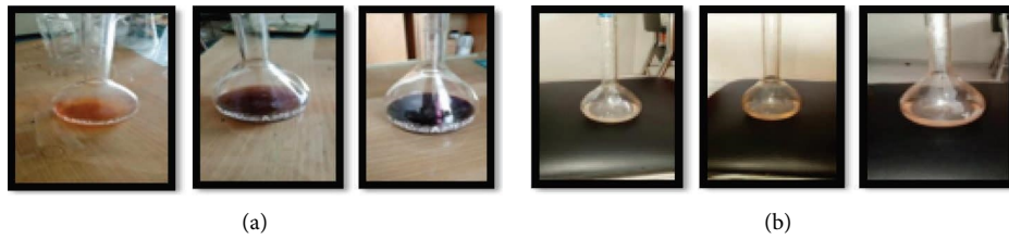
FIGURE 2: Color change in the solution after the addition of (a) PgP extract and (b) PnP due to the reduction of silver ions.
