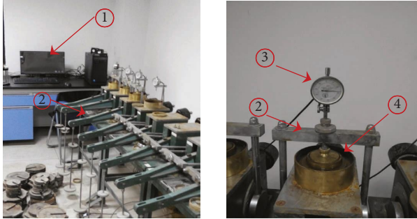
FIGURE 2: The left are the oedometer apparatuses linked with the data auto sampling system. The right is one of the test apparatuses. ① Computer used for indication. ② Loading frame, which can be moved away when measuring the vertical deformation without loading. ③ Dial gauge linking with the computer. ④ Water container, into which a sample is put.
