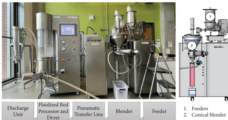
FIGURE 1: Syntegon wet granulation line.
