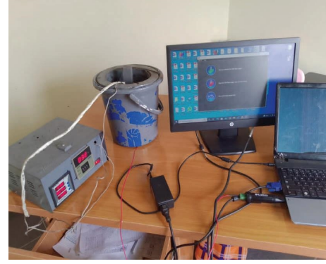
FIGURE 3: Arrangement of sample into the guarded hot plate plugged with the stabiliser.
