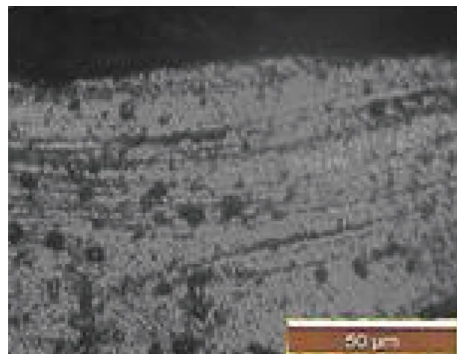
FIGURE 9: Worn surface of the DLC tool.
