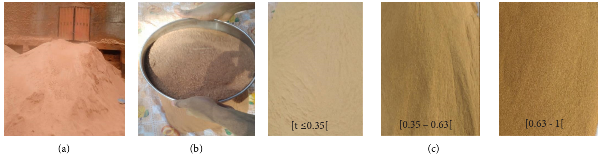
FIGURE 1: Particle size distinction: (a) supply; (b) sieving; and (c) different particle sizes.
