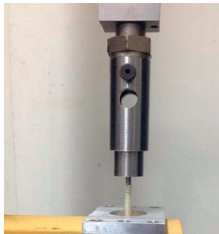
FIGURE 5: Screw axial pull-out strength test performed in compliance with ASTM F 2193 and ASTM F 543 standards using a Testometric M350-10 kN testing machine.
