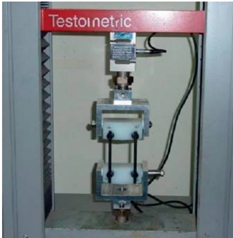
FIGURE 2: Static axial compression bending test performed in compliance with the ASTM F1717 standard, using a Testometric M350-10kN testing machine, and simulating a vertebrectomy model via a large gap between two UHMWPE blocks simulating two vertebrae.
