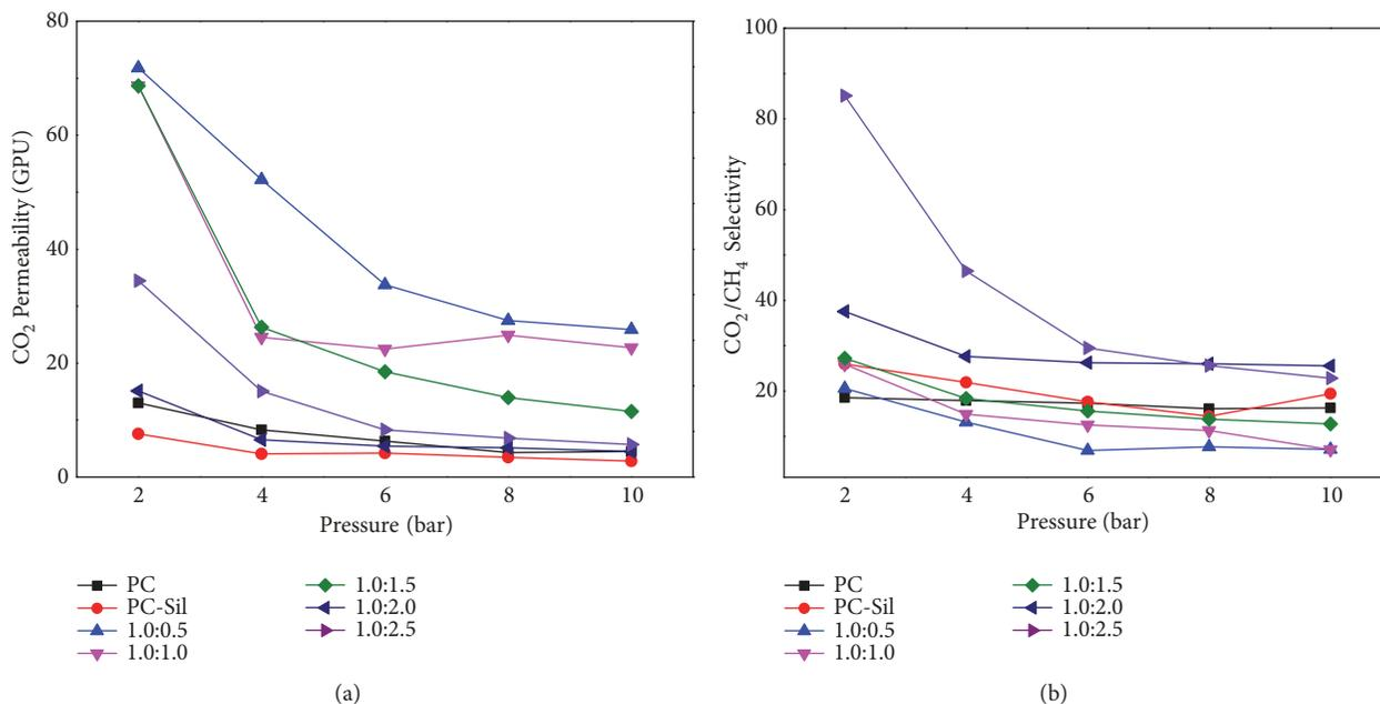
FIGURE 7: Effect of feed pressures on (a)  $\text{CO}_2$  permeance, and (b)  $\text{CO}_2/\text{CH}_4$  selectivity of prepared membranes.
