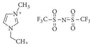
FIGURE 1: Molecular structure of [EMIM][TF<sub>2</sub>N].
