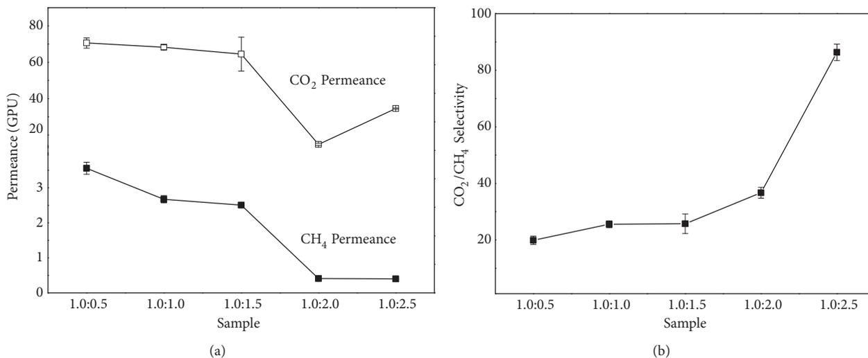
FIGURE 6: Separation performance of PC-Sil-IL at different IL:Si ratio at 2 bar with (a) gas permeance and (b) CO<sub>2</sub>/CH<sub>4</sub> selectivity.
