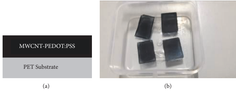
FIGURE 1: (a) Schematic drawing of the thin film side view. (b) Samples of the prepared MWCNT-PEDOT:PSS thin film.
