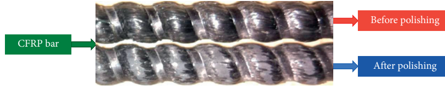
FIGURE 3: Shape of the CFRP bar.
