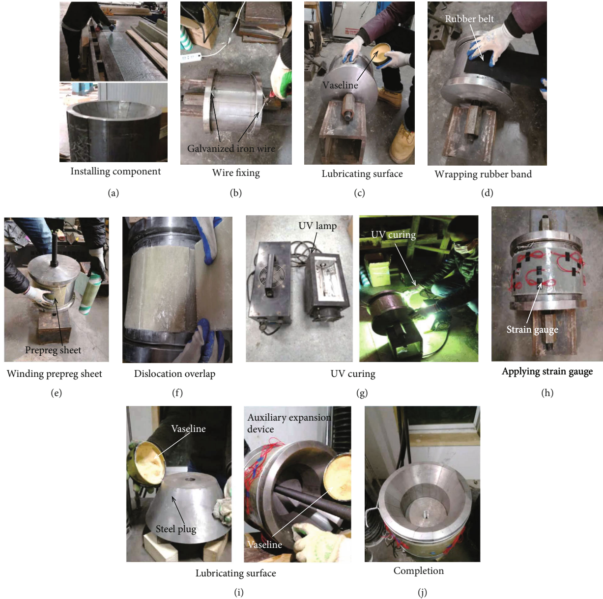
FIGURE 8: The manufacturing process of the specimen: (a) installing component, (b) wire fixing, (c) lubricating surface, (d) wrapping rubber band, (e) winding prepreg sheet, (f) dislocation overlap, (g) UV curing, (h) applying strain gauge, (i) lubricating surface, and (j) completion.
