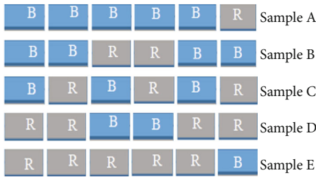
FIGURE 1: The stacking sequence of hybrid composites.
