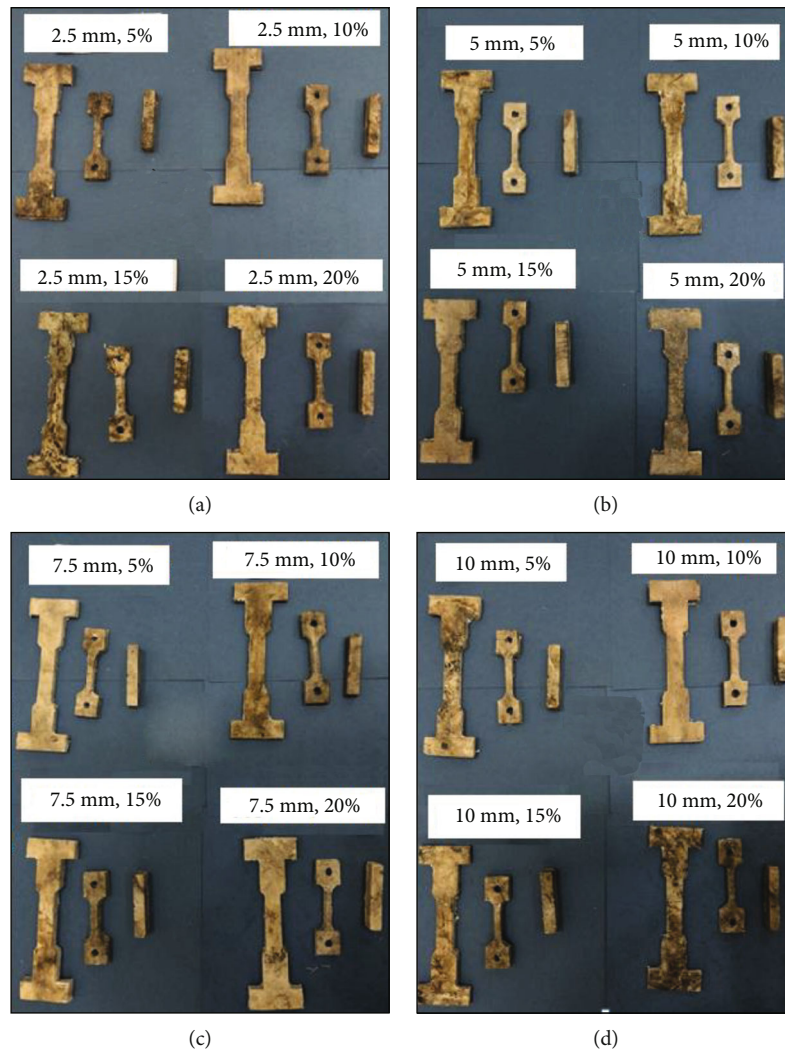
FIGURE 3: Different types of specimens with different lengths and weight ratios of DPF.
