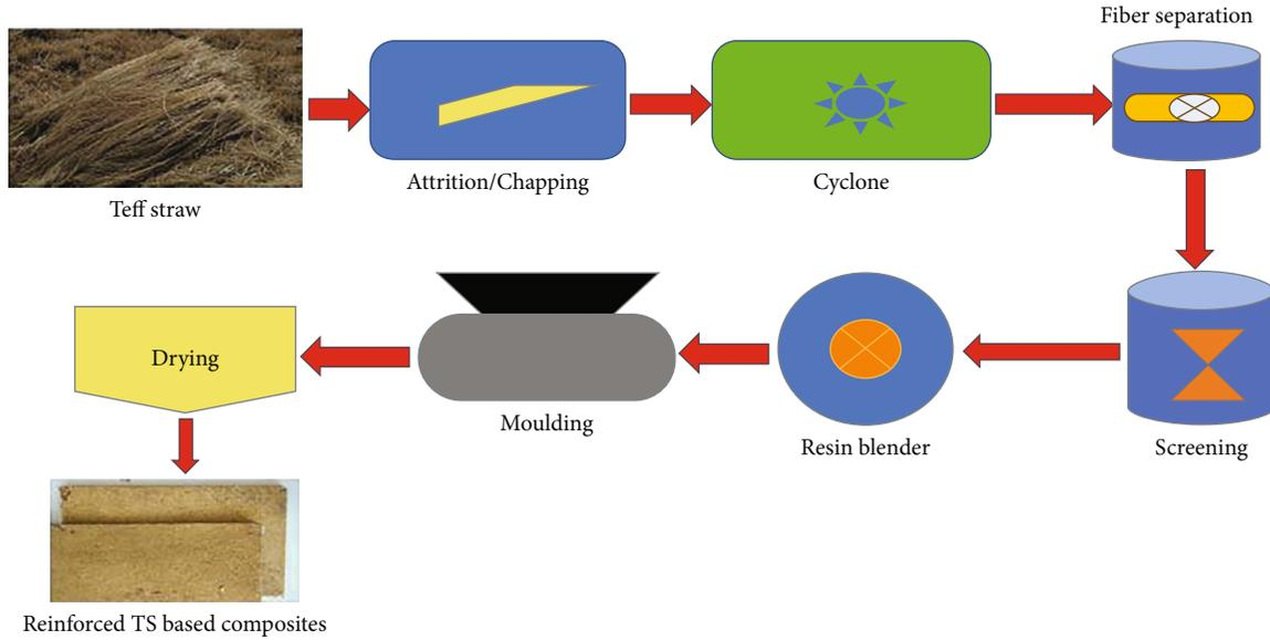
FIGURE 1: Schematic flow of TS-based composite preparation.
