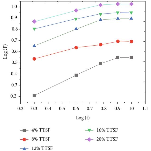
FIGURE 3: The kinetic plot for water absorption on different TTSF fiber loadings of reinforced epoxy composites.
