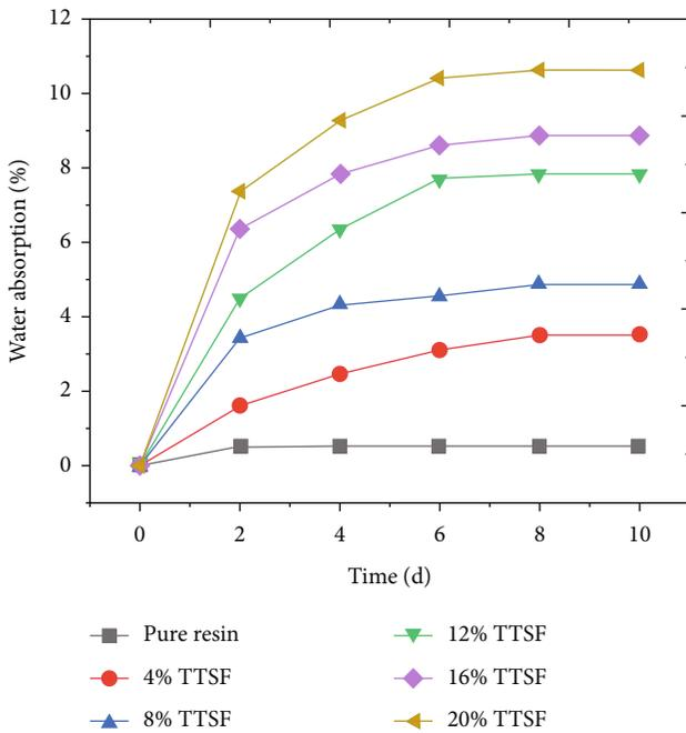
FIGURE 2: The influence of TTSF loading on water absorption for reinforced epoxy composites.
