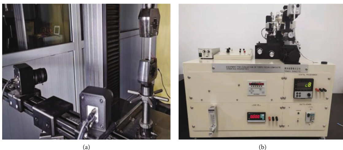
FIGURE 3: The photograph of the test setups (a) Tensile machine and DIC system; (b) composite interface evaluation device.
