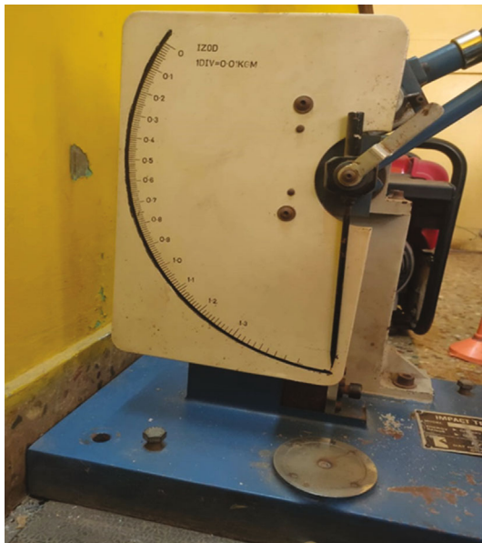
FIGURE 2: Shows the schematic view of impact testing machine.
