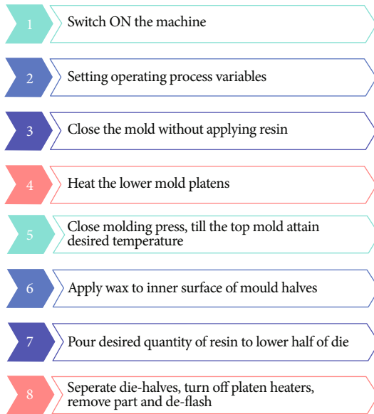
FIGURE 3: Steps involving the compression molding process for producing hybrid composites.
