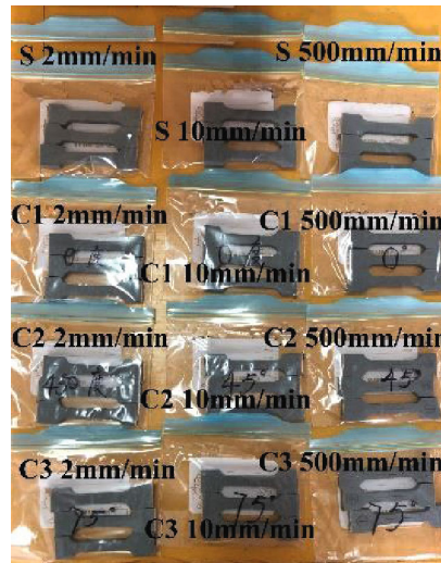
(b) Prefabricated cracked specimen
