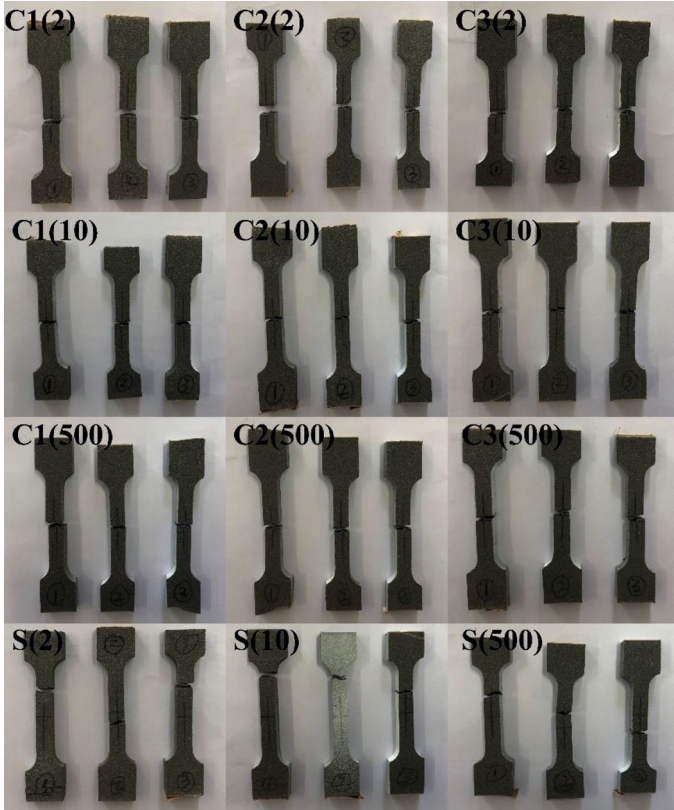
FIGURE 10: Overall shapes of the specimens after fracture.
