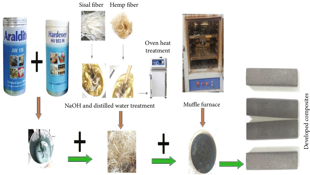
FIGURE 1: Actual flow process fabrication layout for epoxy hybrid nanocomposite.
