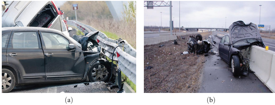
FIGURE 6: Crashes involving vehicles and lane-diving barriers that caused rapid road accidental deaths (a and b).
