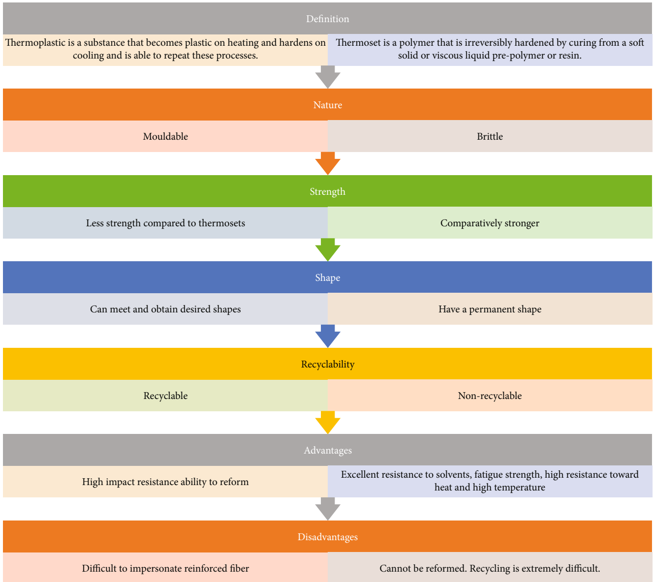
FIGURE 7: Difference between thermoplastic and thermosetting plastics.
