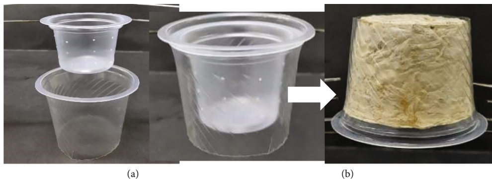
FIGURE 2: Polypropylene plastic cup for biofoam cup casting: (a) before use and (b) after use.
