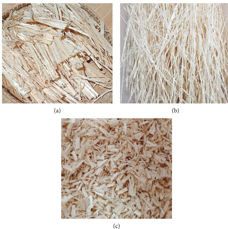
FIGURE 1: (a) Bagasse, (b) depithed bagasse, and (c) bagasse after cutting into small pieces.
