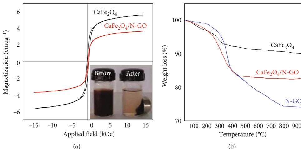
FIGURE 4: Magnetization curve of the synthesized  $\text{CaFe}_2\text{O}_4$  nanoparticles and  $\text{CaFe}_2\text{O}_4/\text{N-GO}$  nanocomposite (inset: the magnetic separation of magnetic nanocomposite after dye removal) (a) and TGA curve of  $\text{CaFe}_2\text{O}_4$  nanoparticles, N-GO, and  $\text{CaFe}_2\text{O}_4/\text{N-GO}$  nanocomposite (b).
