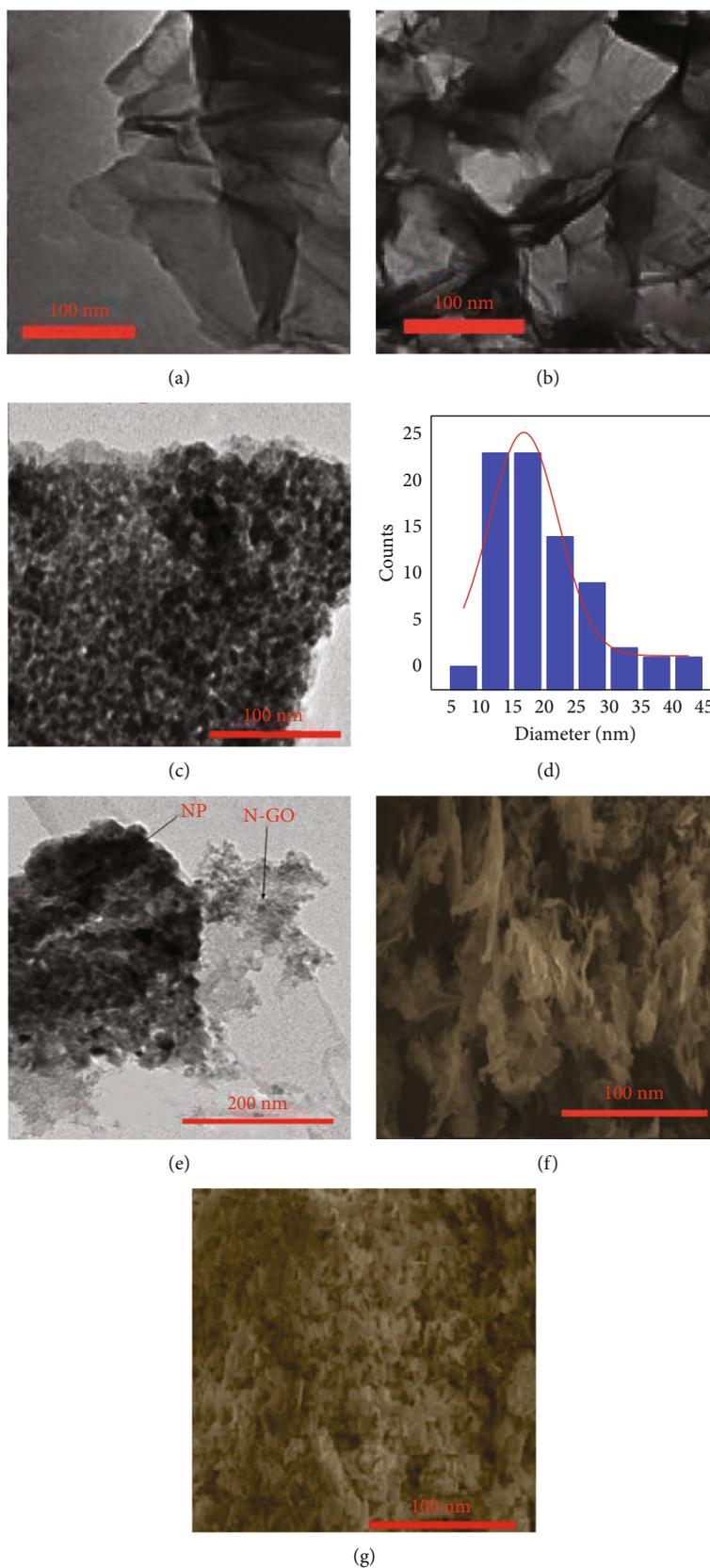
FIGURE 3: TEM images of GO (a), N-GO (b),  $\text{CaFe}_2\text{O}_4$  nanoparticles (c),  $\text{CaFe}_2\text{O}_4$  nanoparticles size histogram (d),  $\text{CaFe}_2\text{O}_4$ /N-GO nanocomposite (e), SEM images of  $\text{CaFe}_2\text{O}_4$  nanoparticles (f), and  $\text{CaFe}_2\text{O}_4$ /N-GO nanocomposite (g).
