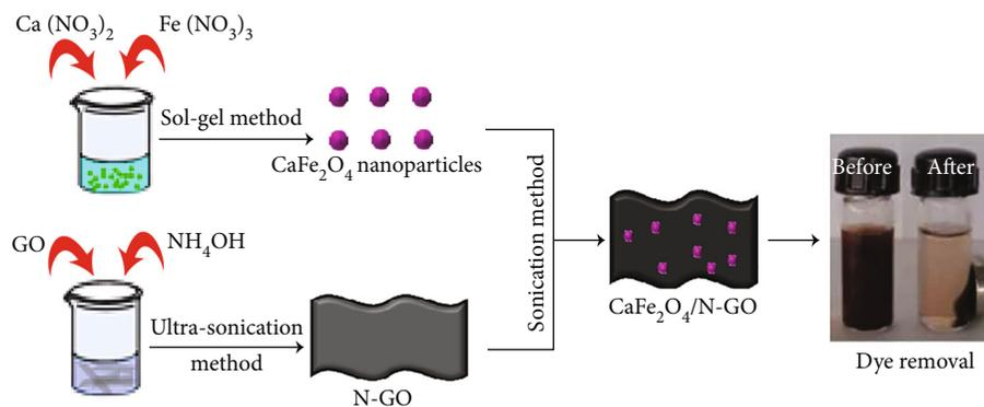
FIGURE 1: Schematic diagram for the synthesis  $\text{CaFe}_2\text{O}_4/\text{N-GO}$  nanocomposite.
