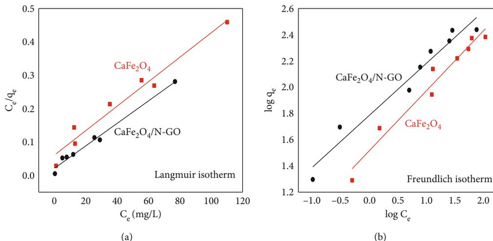
FIGURE 8: Fitting the experimental data to Langmuir isotherm model (a) and Freundlich isotherm model (b) for the adsorption of RO12 dye on the surface of  $\text{CaFe}_2\text{O}_4$  nanoparticles and  $\text{CaFe}_2\text{O}_4/\text{N-GO}$  nanocomposite.
