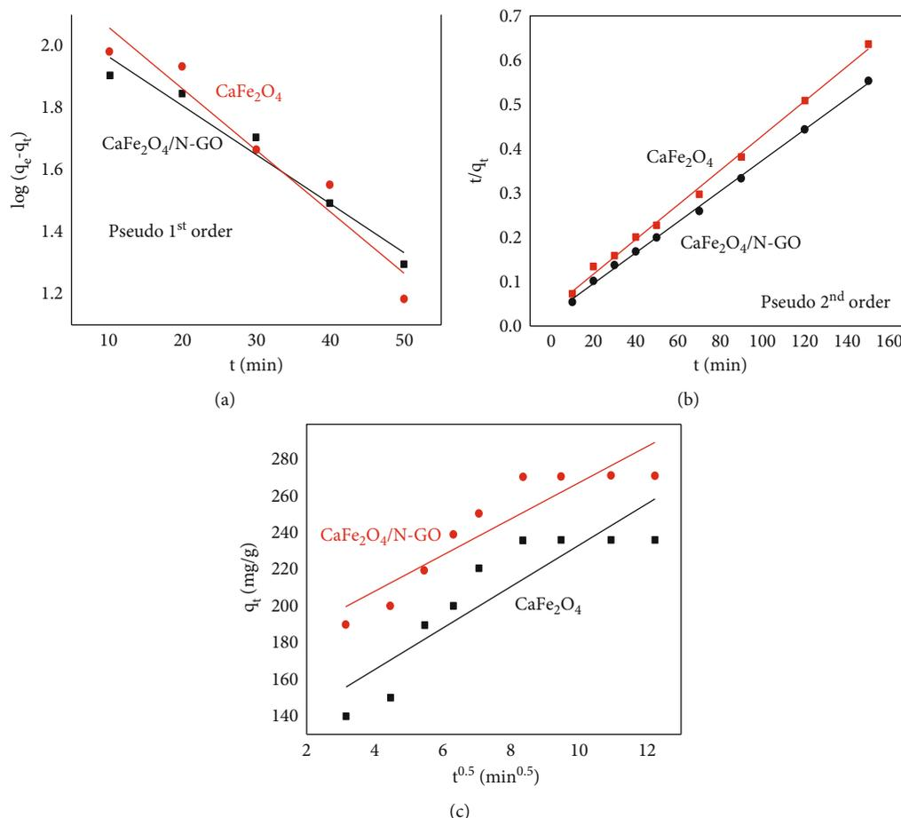
FIGURE 7: Fitting the experimental data to pseudo 1<sup>st</sup> order kinetics (a), pseudo 2<sup>nd</sup> order kinetics (b), and intraparticle diffusion model (c) for the adsorption of RO12 dye on the surface of  $\text{CaFe}_2\text{O}_4$  nanoparticles and  $\text{CaFe}_2\text{O}_4/\text{N-GO}$  nanocomposite.
