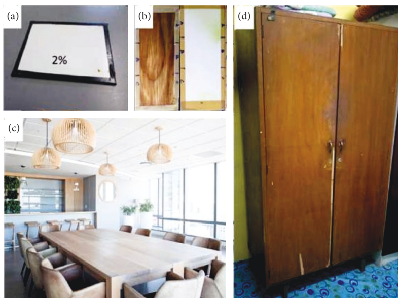
FIGURE 18: Different surfaces coated with paint containing ZnO NPs. (a) Carbon steel surface coated with paint blended with 2% ZnO NPs, (b) clear PU and white PU blended with ZnO NPs for wood and cement slab panels, respectively, (c) and (d) display common wood used in households. The image was taken from Ref. [23].
