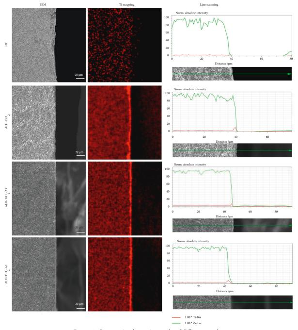
Figure 2: Cross-sectional mapping results of different samples.
