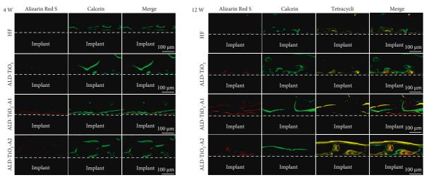
FIGURE 9: Polychrome sequential fluorescent labels at 4 weeks and 12 weeks after implantation in rat femoral condyle models: 4 weeks (a) Alizarin Red S (red, 1 week) and calcein (green, 3 weeks); 12 weeks (b) Alizarin Red S (red, 4 weeks), calcein (green, 8 weeks), and tetracycline hydrochloride (yellow, 11 weeks).
