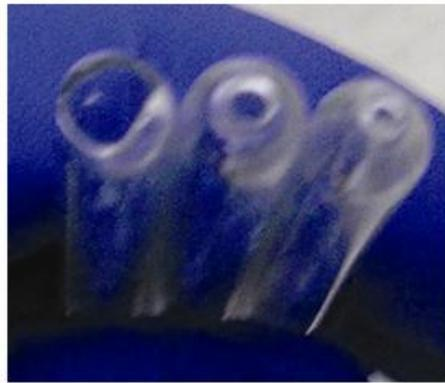
**Supplemental Figure 3: Trituration Pipettes.** From left to right: Large bore, useful for samples containing pieces of bone; medium bore, useful for fragile samples free of bone (soleus, deboned intercostal); small bore, used only for short muscle fibers/small cells (FDB, non muscle tissue).
