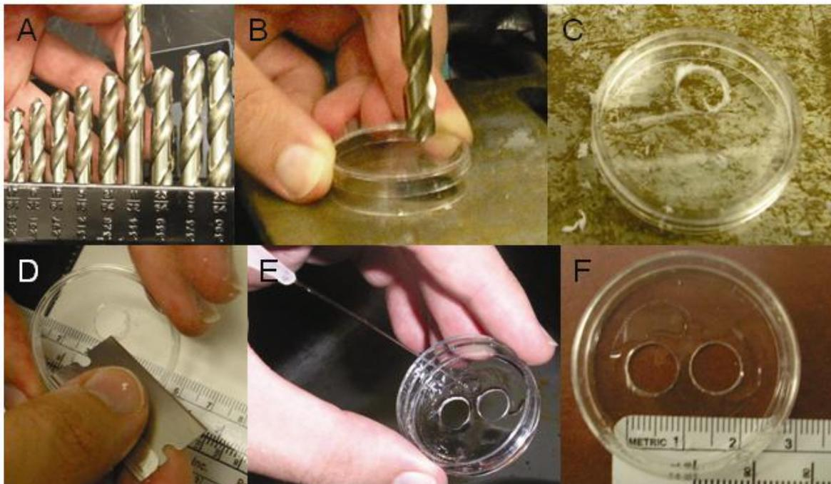
**Supplemental Figure 1: Drilling Wells.** An  $1\frac{1}{32}$ " bit (A) was used to drill the bottom face of a 35mm Falcon Petri dish (B). This configuration results in the plastic burr on the outside of the dish (C) where it can easily be removed (D). Following burr removal dishes are washed in 70% ethanol (E). If increased plating area is desired, extra wells may be drilled (F) rather than increasing the diameter.
