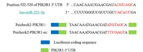
Supplemental Figure 1. A schematic diagram showing the construction of the luciferase reporter vectors
