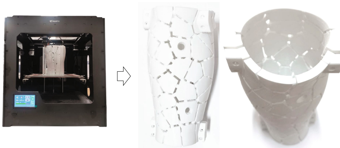
FIGURE 9: Manufacturing of the external fixator through 3D printing.
