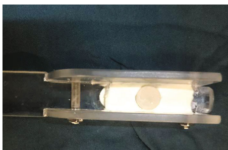
FIGURE 3: Sample prepared for placement in the brushing simulator.
