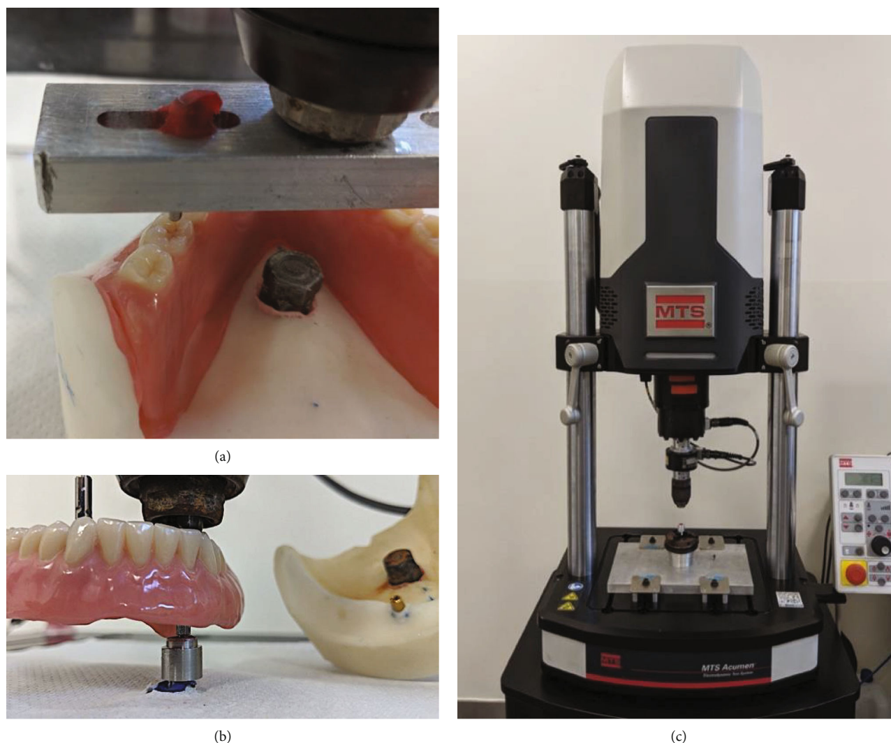
FIGURE 3: A) Engagement of the first molar; B) Retention test setting; C) MTS Acumen.
