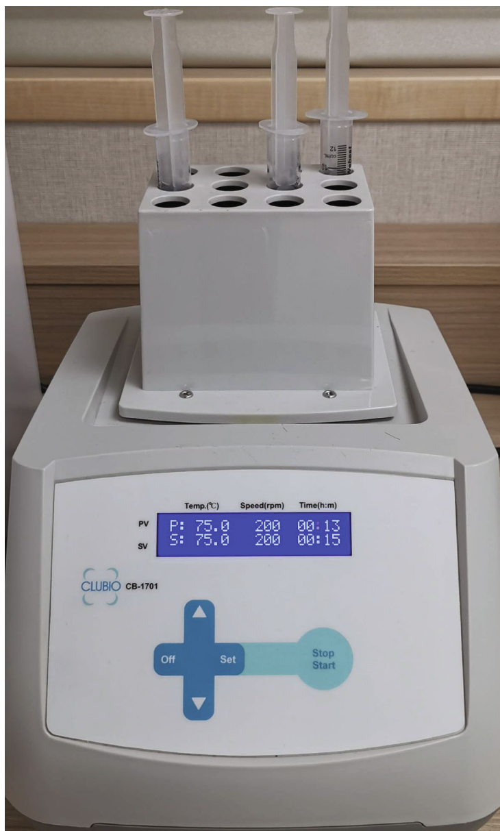
FIGURE 1: The thermal oscillation technique (machine set at 75 degrees Celsius and under an oscillation speed of 200 revolutions per minute for a total of 15 minutes). Syringe containing the liquid-form PRP was placed into the machine chamber for thermal oscillation. Airtightness is ensured by using the 10 mL syringe.
