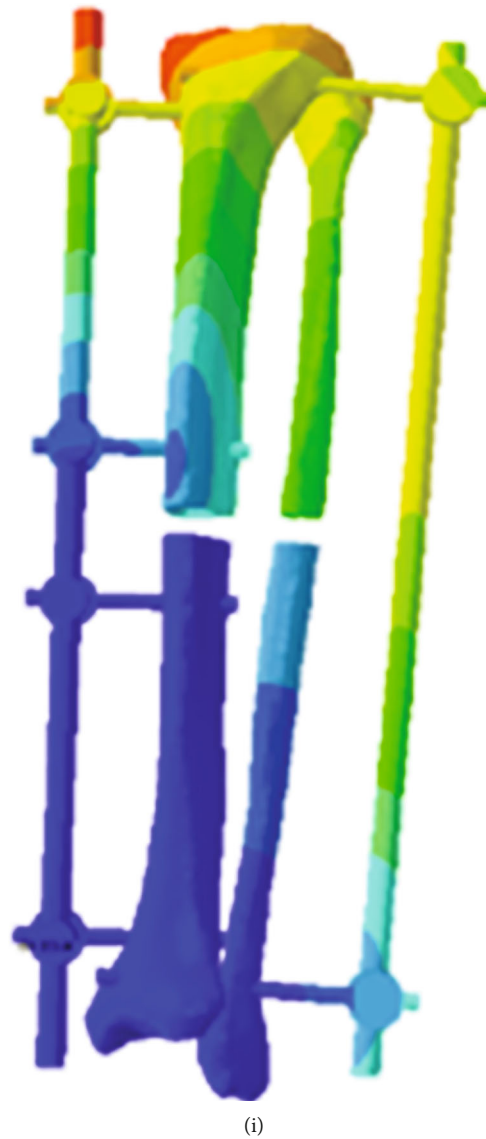
FIGURE 4: Maximum displacements of 9 configurations under vertical load. (a) 2.199 mm. (b) 2.165 mm. (c) 5.672 mm. (d) 4.963 mm. (e) 2.294 mm. (f) 2.063 mm. (g) 2.048 mm. (h) 1.508 mm. (i) 0.673 mm.
