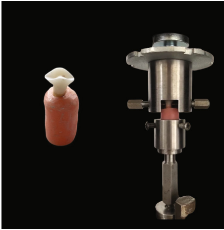
FIGURE 2: The MZ crown specimen and the tensile bond strength test.
