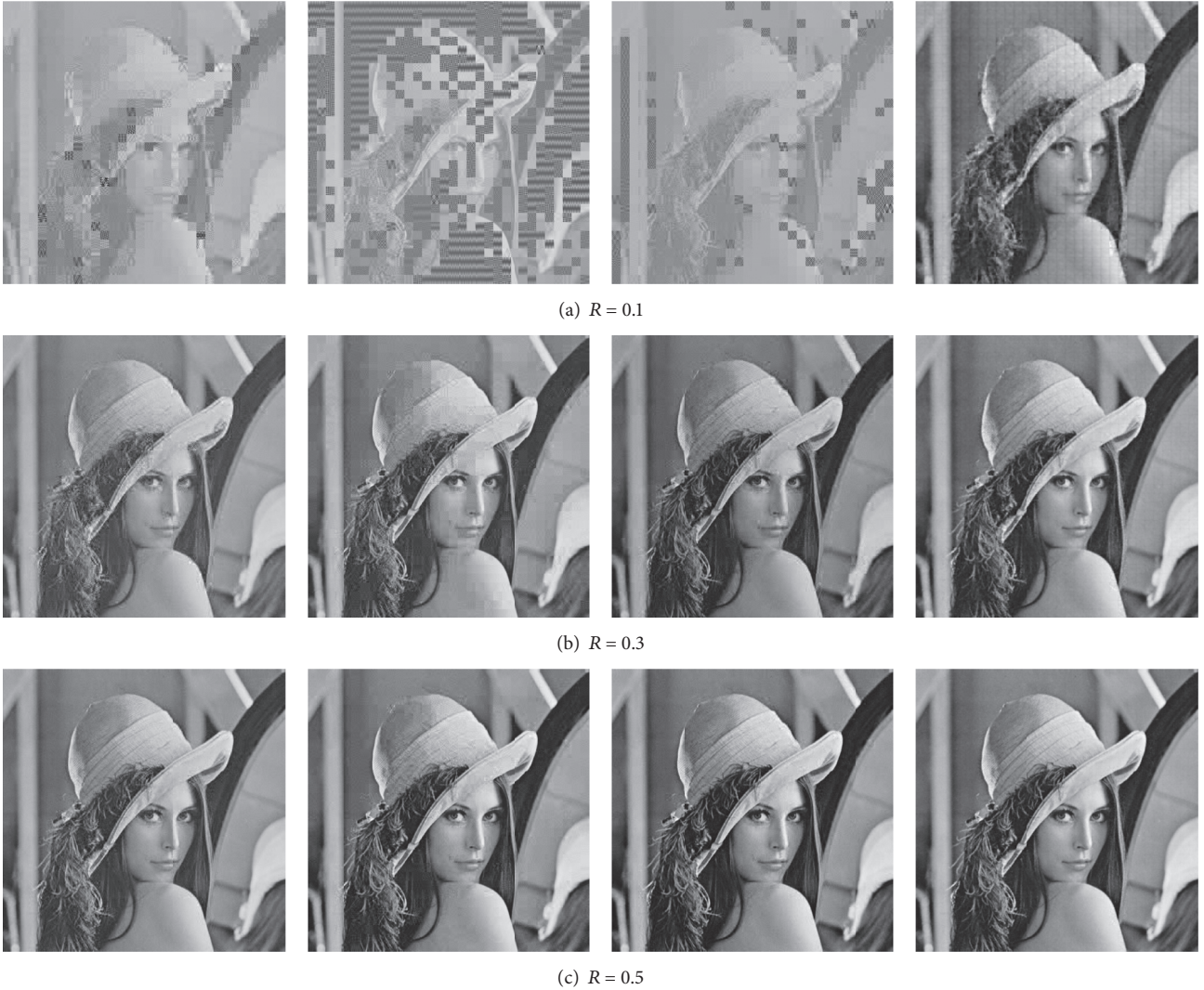
FIGURE 3: Subjective comparison of reconstructed Lenna images by various CS-based codec at different measurement rates. From left to right: BCS, V-ABCS, S-ABCS, and the proposed ABCS. Note that R is the total measurement rate.
