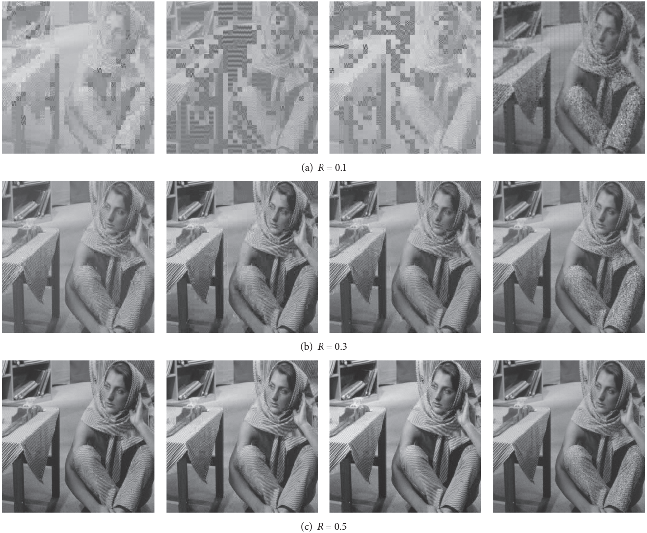
FIGURE 4: Subjective comparison of reconstructed Barbara images by various CS-based codec at different measurement rates. From left to right: BCS, V-ABCS, S-ABCS, and the proposed ABCS. Note that R is the total measurement rate.
