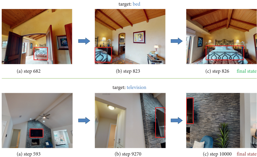
FIGURE 2: An example of exploring processes with two kinds of termination condition. The episode of navigating to bed ends when the agent observes the target clearly at the nearest viewpoint. Since in the other exploring process the agent fails to gain the full view of the television, the training episode is terminated at step 10,000.
