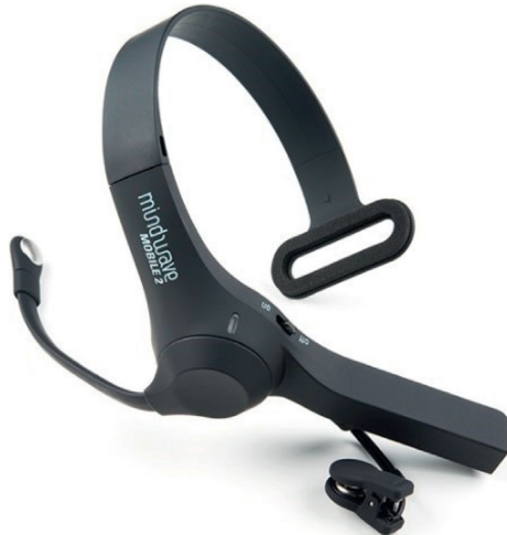
FIGURE 2: Single-channel NeuroSky MindWave mobile 2.
