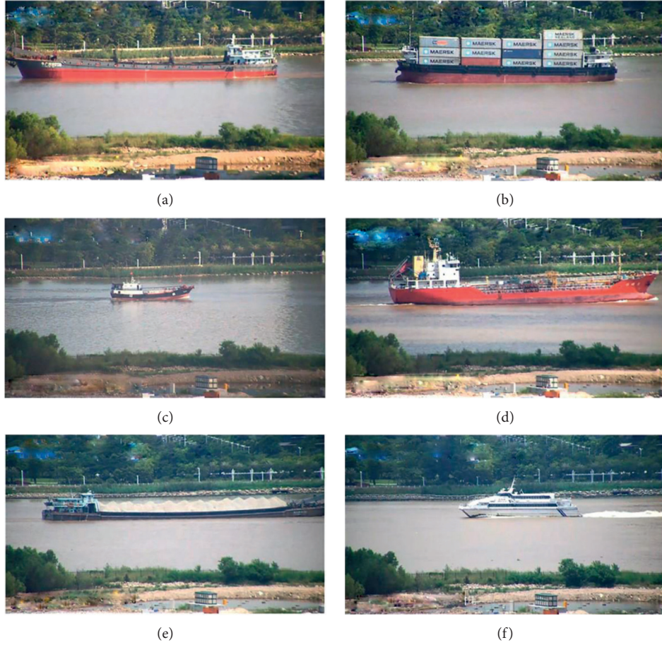
FIGURE 10: The ship category in our used dataset. (a) Bulk cargo carrier. (b) Container ship. (c) Fishing boat. (d) General cargo ship. (e) Ore carrier. (f) Passenger ship.
