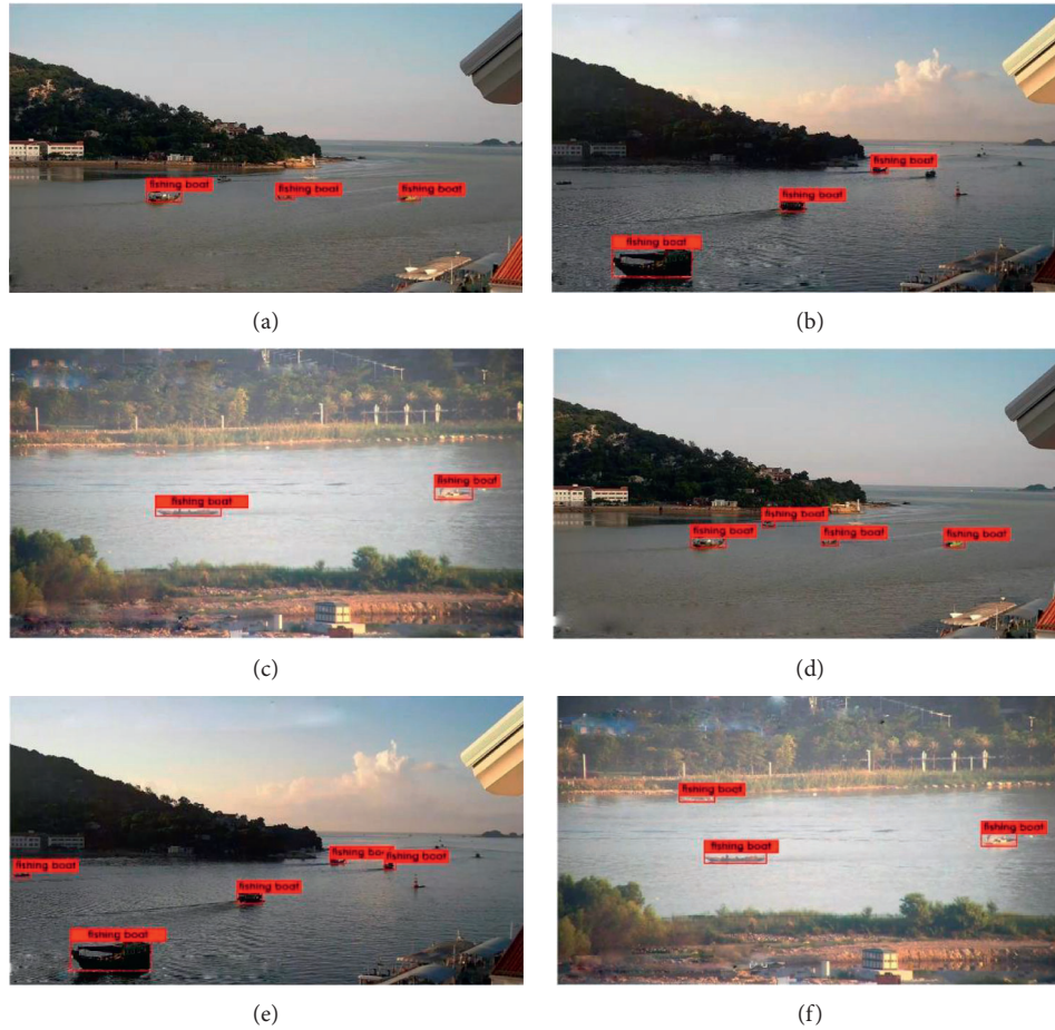
FIGURE 12: Some fishing boats' detection results. (a-c) The original SSD. (d-f) Our proposed method.
