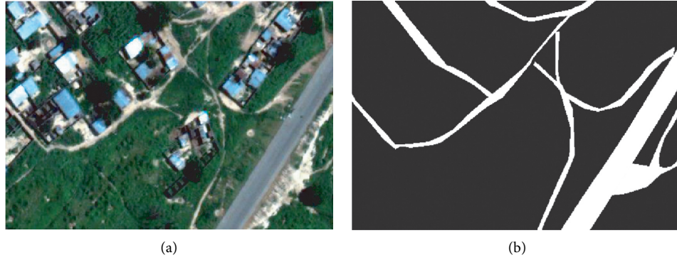
FIGURE 2: Illustration of road mask extraction in remote sensing images. (a) Original image. (b) Extracted road mask.
