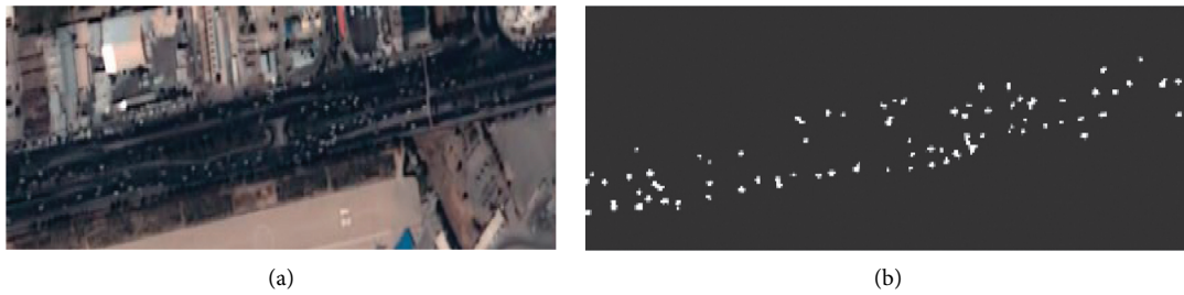
FIGURE 3: Illustration of moving targets detection in the remote sensing video. (a) Remote sensing image. (b) Detection results of moving targets.
