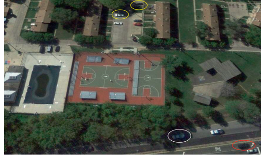
FIGURE 2: The car category in the remote sensing dataset. Where targets marked by yellow circles are vehicle targets obscured by trees, target marked by the white circle is vehicle target in shadow, and target marked by the red circle is vehicle target whose color is similar to that of the surrounding environment.
