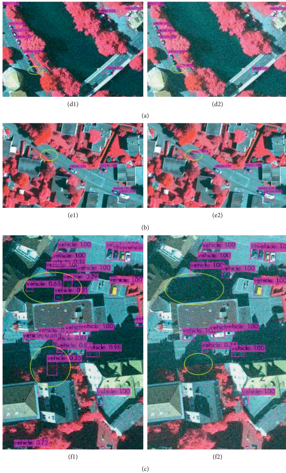
FIGURE 10: The results of dark target detection are compared, where (a, c, e) are the detection results of YOLOv4 and (b, d, f) are the detection results of IR-PANet, where the comparison results of (e and f) can see that YOLOv4 is easier to identify the shadow block as a target, while IR-PANet is more accurate.
