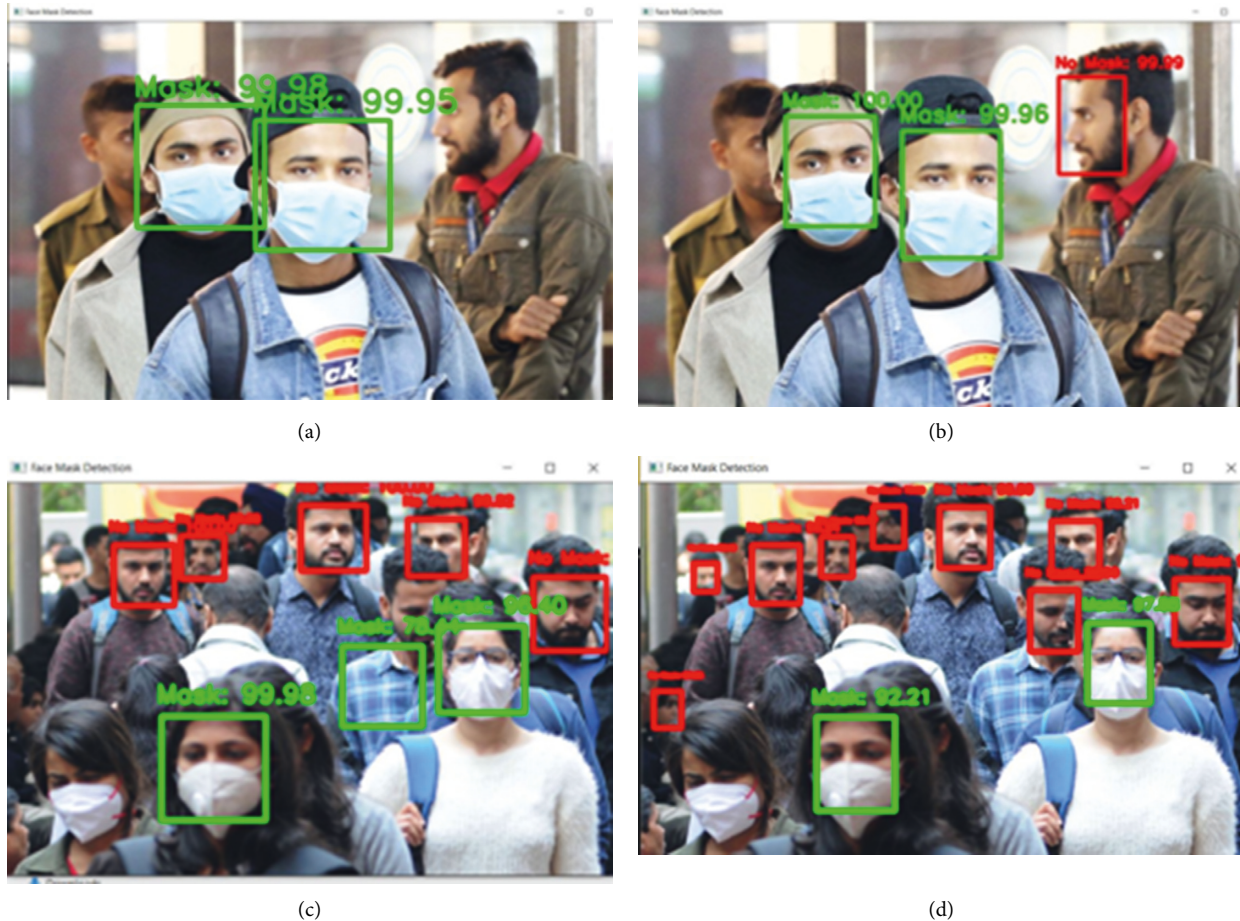
FIGURE 7: (a) Haar Cascade not able to detect side faces. (b) MTCNN able to detect side faces. (c) False positive with Haar Cascade. (d) No false positive with MTCNN.
