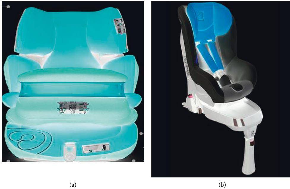
FIGURE 6: Physical simulation of the child seat. (a) Front-guard-type CRS. (b) Strap-type CRS.
