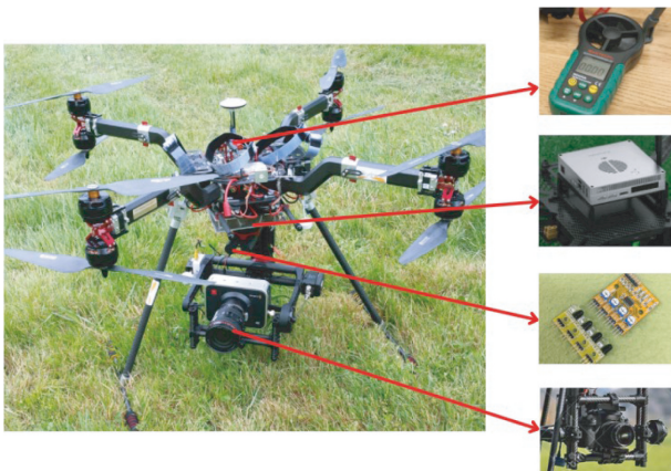
FIGURE 4: Digital anemometer manifold with CPU, IR sensors, and 12k camera.
