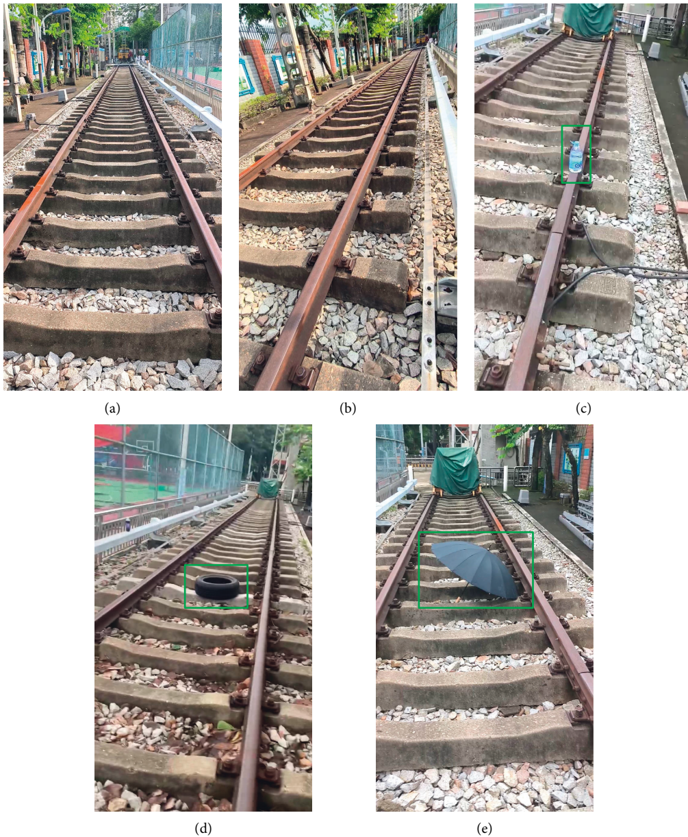
FIGURE 8: Illustration examples of the railway foreign object dataset. (a, b) Normal railway images. (c–e) Intruded railway images with corresponding reference bounding boxes (green) of the objects.
