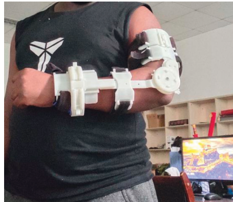
FIGURE 9: SEB was worn by a participant to test ROM and to use it for serious game rehabilitation.
