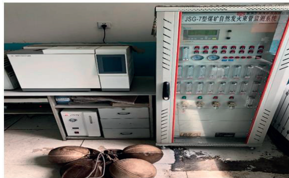
FIGURE 3: Ground beam tube analysis device.
