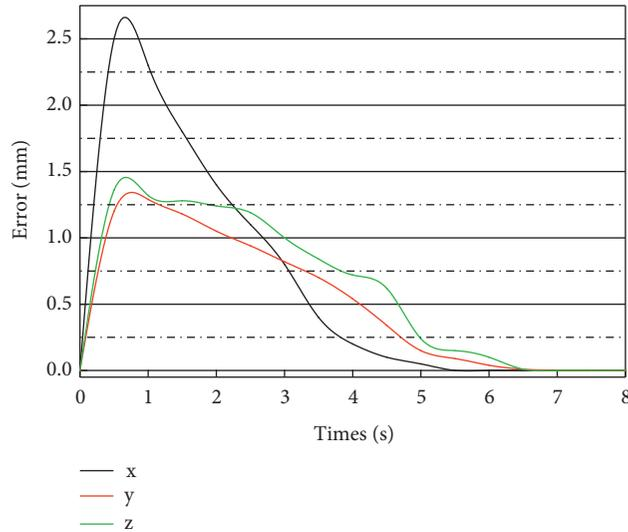
FIGURE 5: TCP position error using a controller.
