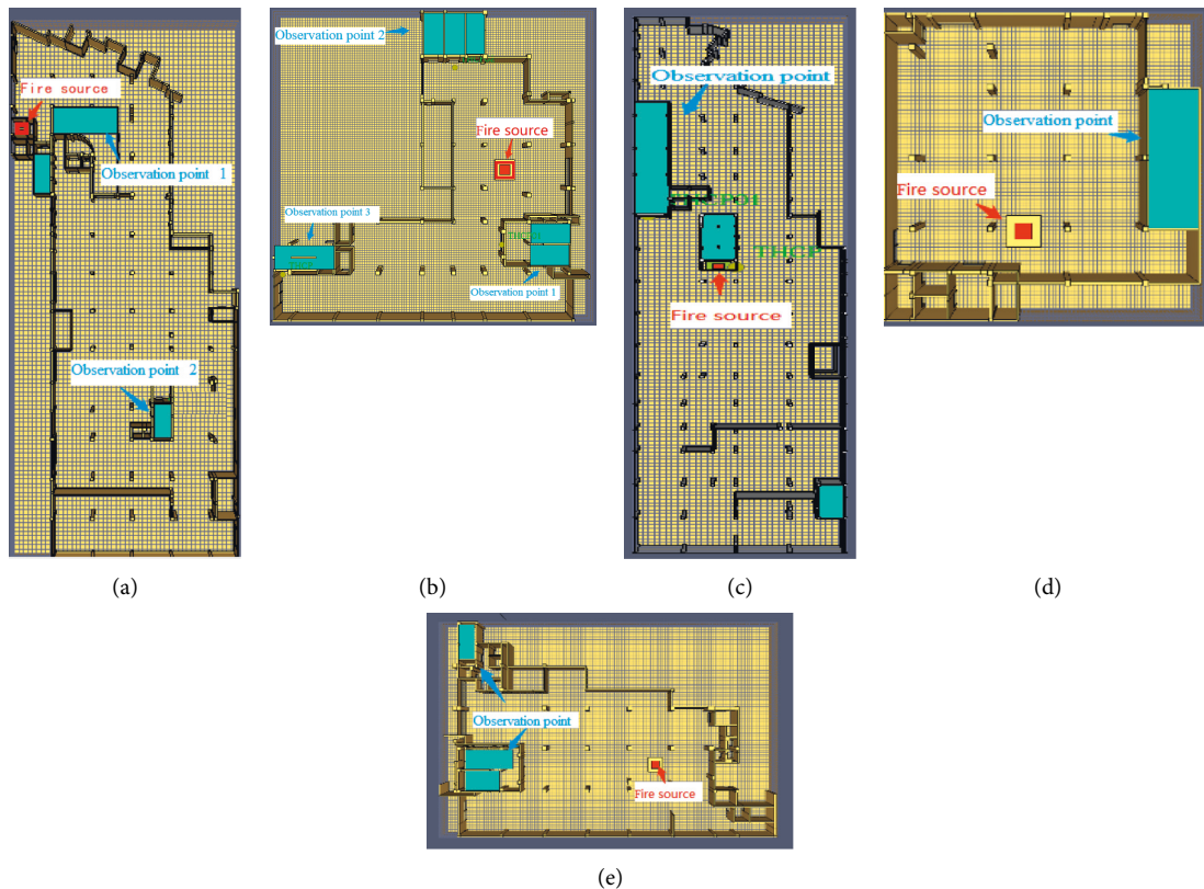
FIGURE 3: Schematic diagram of fire source locations in a different scenario: H1–H5. (a) Schematic diagram of fire source location H1; (b) schematic diagram of fire source location H2; (c) schematic diagram of fire source location H3; (d) schematic diagram of fire source location H4; and (e) schematic diagram of fire source location H5.
