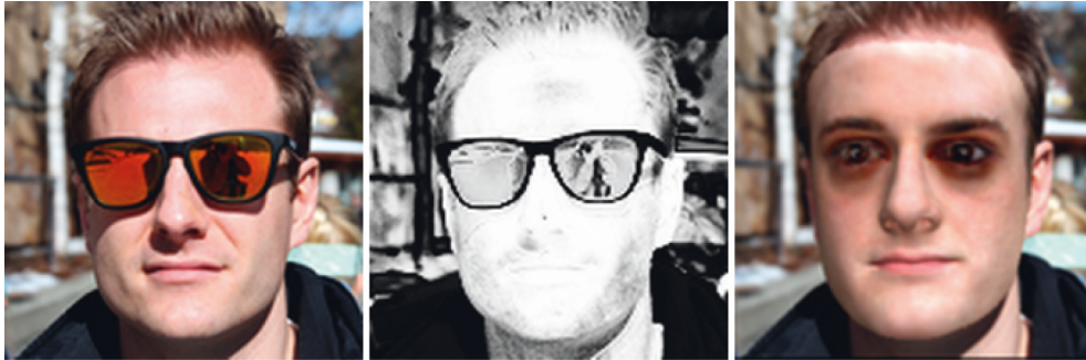
FIGURE 2: The shadow problem brought by using only spatial domain loss: in the mask map (middle), we found that when the occlusion color is complex, the mask is correspondingly not good, so it will lead to the phenomenon of “under-eye dark circle” (right).
