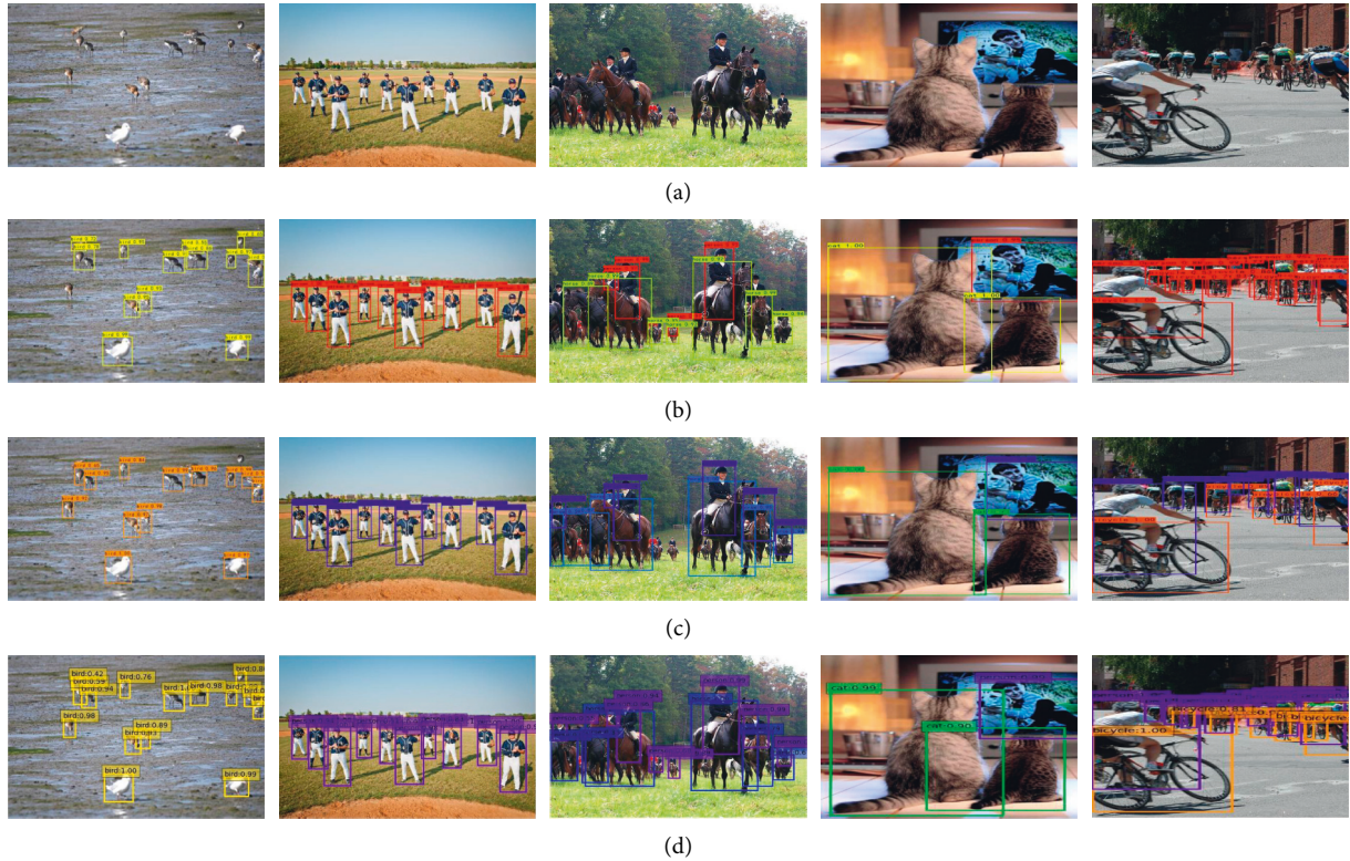
FIGURE 5: Qualitative test results on MS COCO2017: (a) image, (b) YOLOv3, (c) YOLOv4, and (d) FIEN512.
