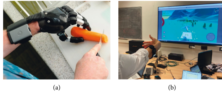
FIGURE 1: Applications of myoelectric pattern recognition. (a) Prosthetic hand source: https://mcoopro.com/blog/resources/arm-hand-prosthetics/ (accessed on 05 Apr. 2022). (b) Game controller (source: https://www.miro.ing.unitn.it/emg-remote-control-of-a/ ) (accessed on 05 Apr. 2022).
